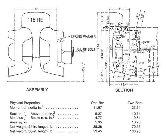
Figure 4-3-1. Joint Bar Assembly for 115 RE and 119 RE Rail (115 RE shown)<sup>1</sup>
