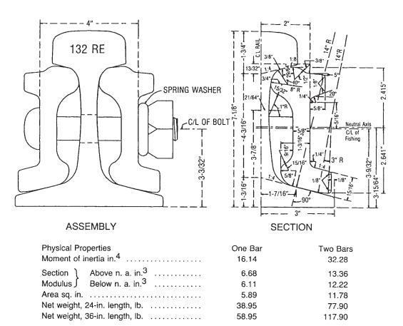
Figure 4-3-3. Joint Bar and Assembly for 132 RE, 136 RE and 141 RE Rail (132 RE Shown)<sup>1</sup>
